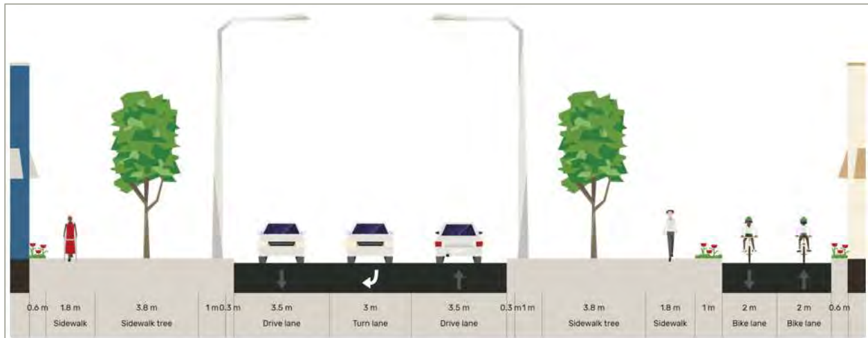
Exhibit 5-24: Typical Cross-Section, 30m Type C Arterial with Regional Trail
